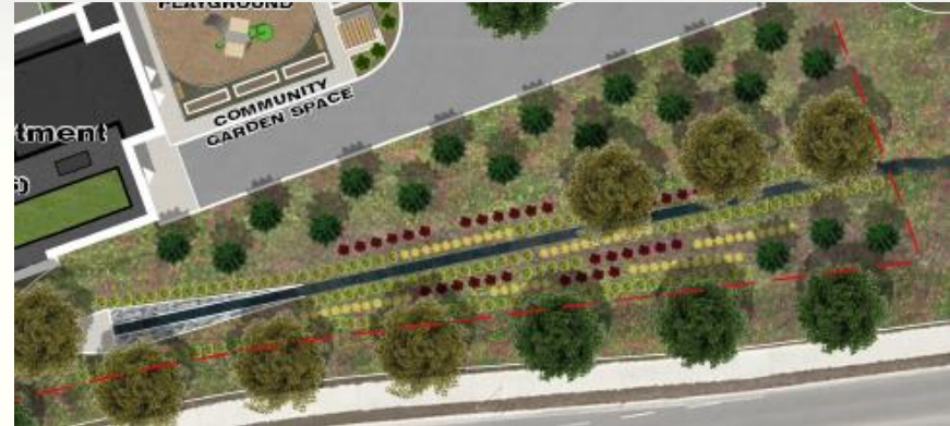
Image: drainage channel re-alignment and watercourse enhancement
