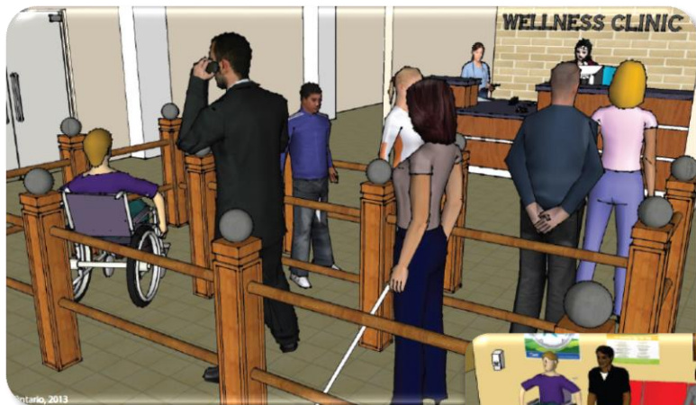
Accessible fixed queuing guides
