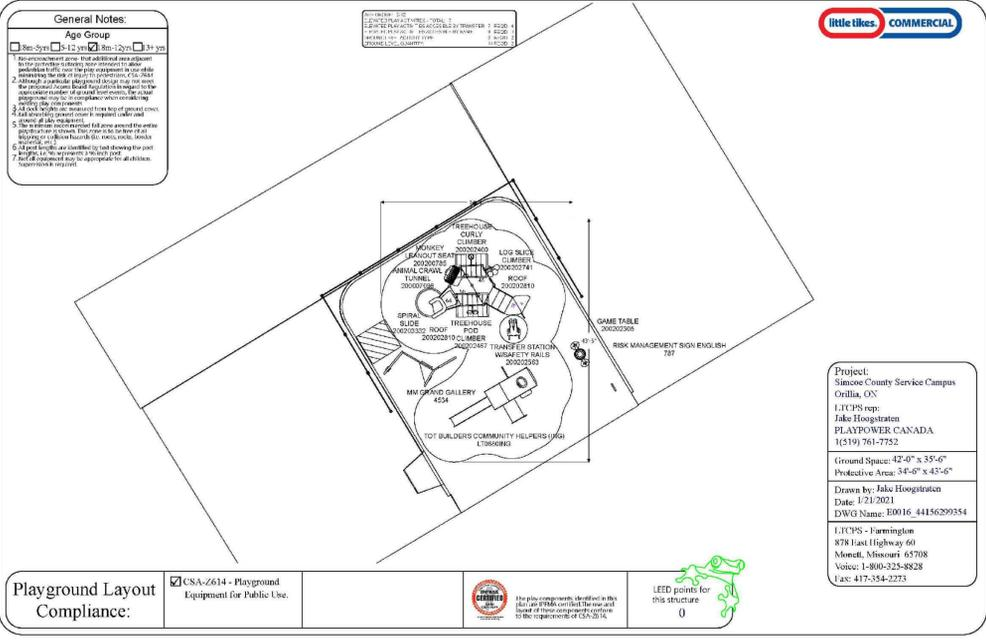
NOTE: ALL TOYS AND EQUIPMENTS TO BE INSTALLED ON CONCRETE FOOTINGS UNDER THE SUPERVISION OF THE LANDSCAPE ARCHITECT. REFER TO THE MANUFACTURER'S SPECIFICATIONS.
