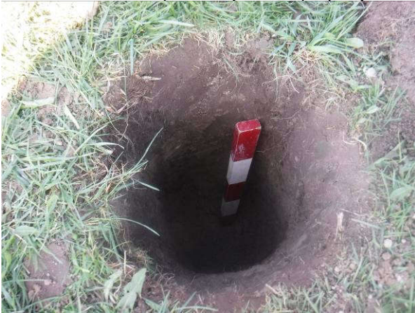
Plate 11: Example of test pit with disturbed soil profile with layer of concrete at bottom.
